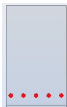
Fig. 5.2 Reinforcement (5φ20) assumed in [1]
